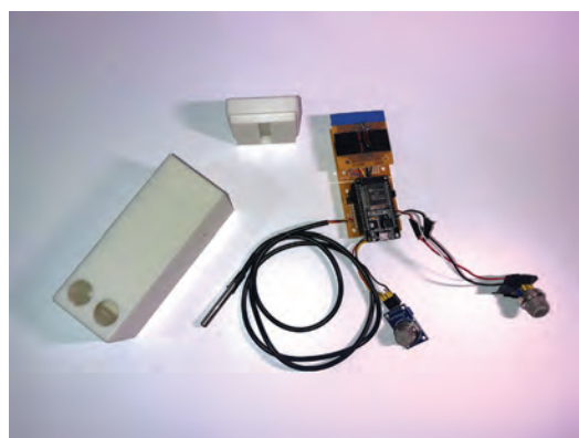
MUDBUG's sensor prototype is designed to remotely monitor soil quality.
